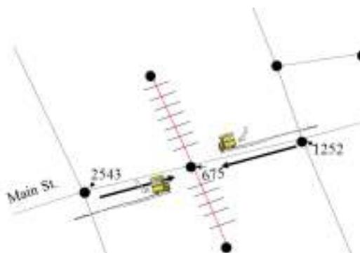
**NOTE:** Problems can exist if stops exist on the segment that has a railroad-crossing node attached, therefore, the segment will need to be split and a new node created.
